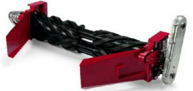
The job of the conditioner is to press and split the fodder; this opens the outer waxy layer of the stems so that the excess water flows out, thus accelerating the drying process, while maintaining the body and all the nutritional elements. In the 4-drum mowers, the conditioner with helical rubber rollers (Chevron type) features a central separator which gives the row a precise form and controls the fodder flow.
